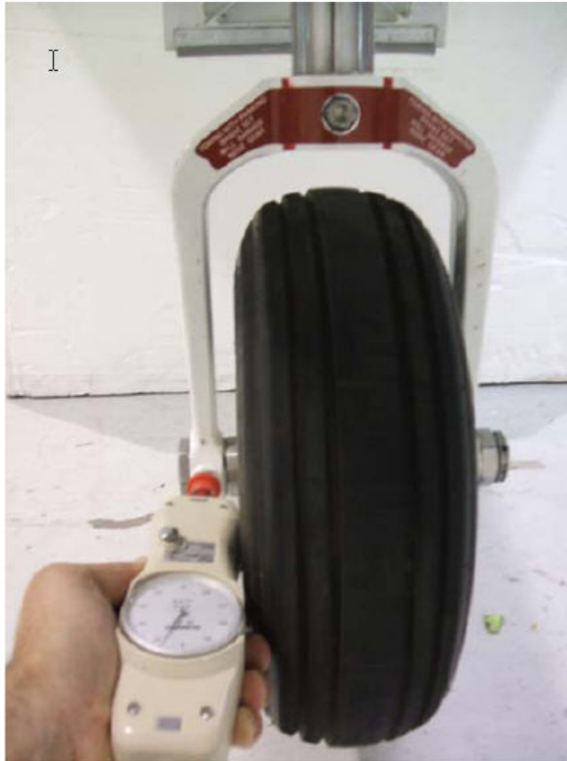
Push-Pull Gauge Application to NLG Figure 1 (Sheet 1 of 1)
